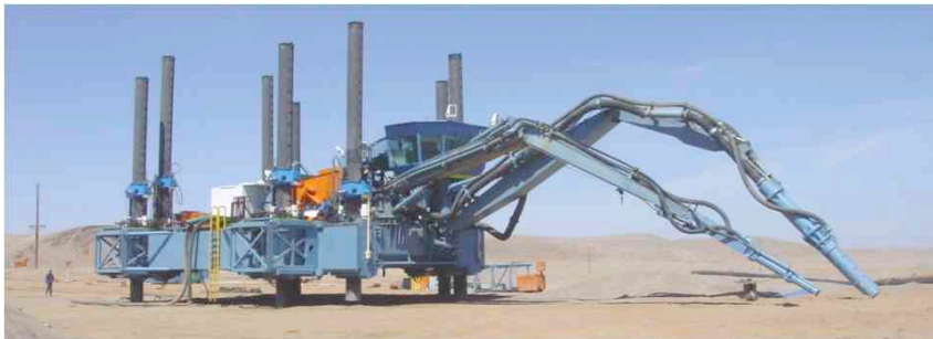
Jet rig used to recover diamond in shallow water. Photo from Namdeb Company brochure.
